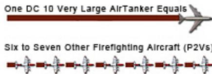
*One DC-10 drop equals the drops of six to seven P2Vs.*
